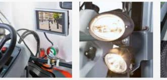
Big cabin windows, a lighting system with integrated work light as a standard and an optional rear view monitor ensure a panoramic all-round view for increased safety.
