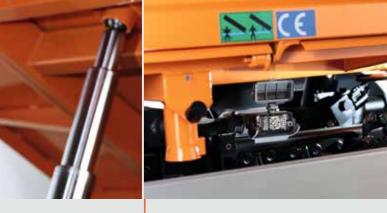
Detachable interface between the tipping cylinder and the tipper.
