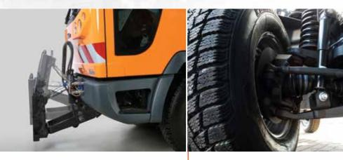
Front lift with attachment plate for easy mounting of attachments – tool-changing quickly accomplished.
