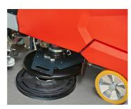
Rapid brush changing: The automatic discharge and pickup system provides rapid and comfortable changing of the brushes.
