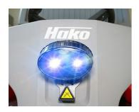
Increased safety in aisles: The BlueSpot head lamp signals an oncoming vehicle.
